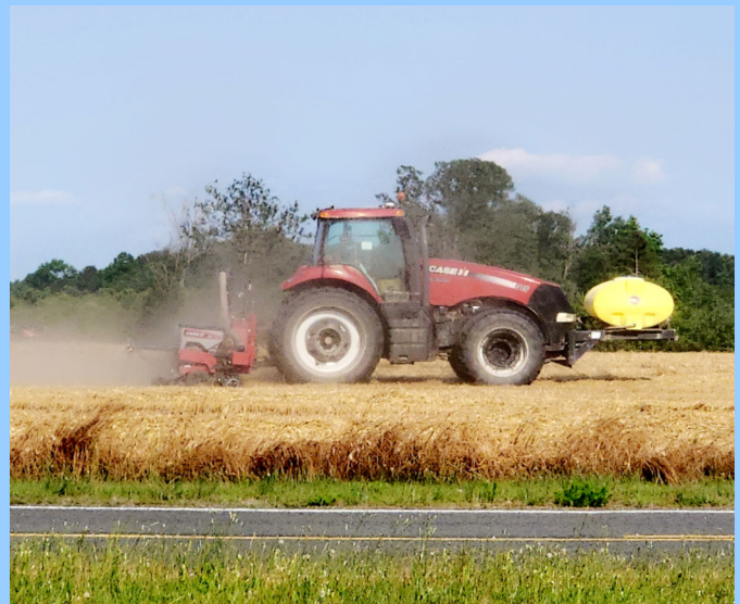
No-till planting into a terminated cover crop
